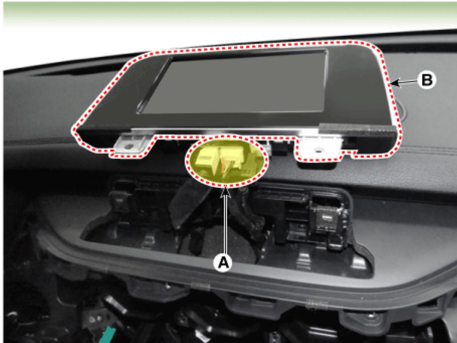
33. Remove the monitor fascia panel (A) after loosening the mounting screws.
