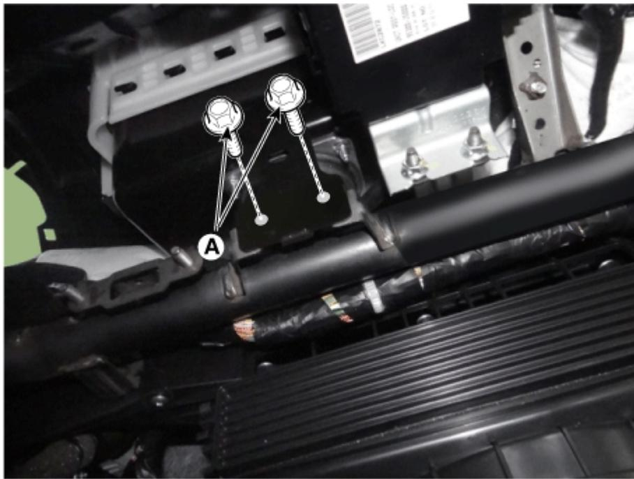
41. Separate the main crash pad assembly (A) after loosening the mounting bolts and nuts.
