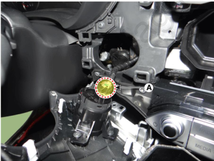
15. Remove the cluster fascia panel (A) by using a remover.
