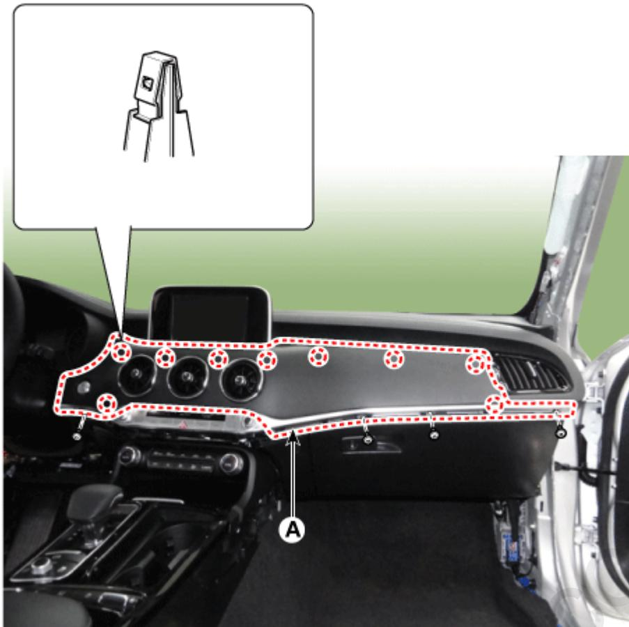
14. Disconnect the start/stop button connector (A) and then remove the crash pad garnish.
