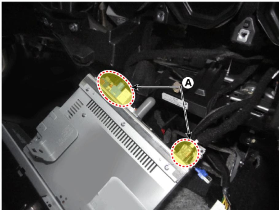
31. Separate the monitor assembly (A) after loosening the mounting screws.
