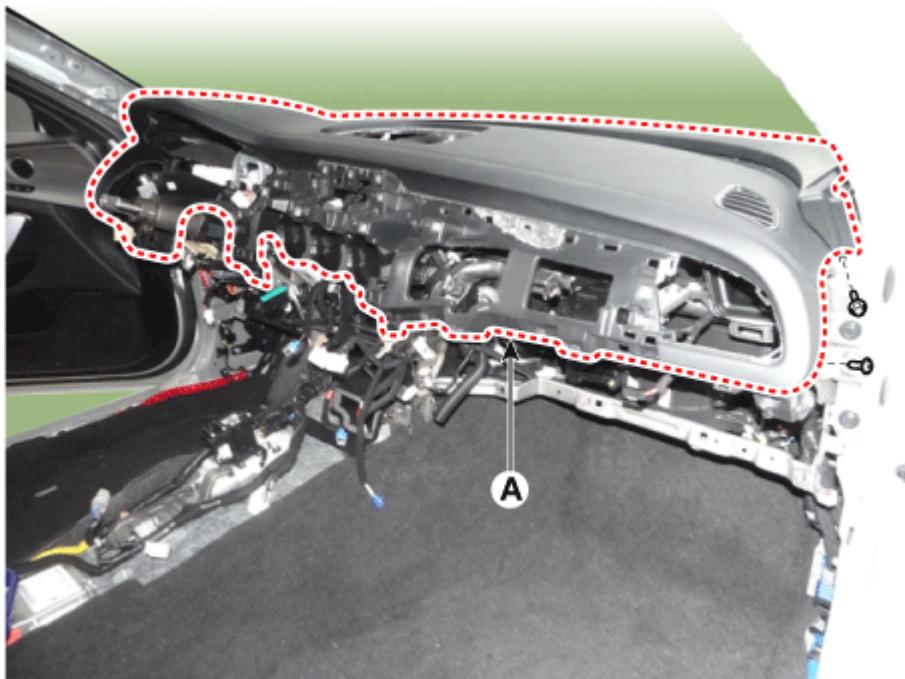
42. Remove the crash pad assembly after disconnecting the passenger airbag connector (A).
