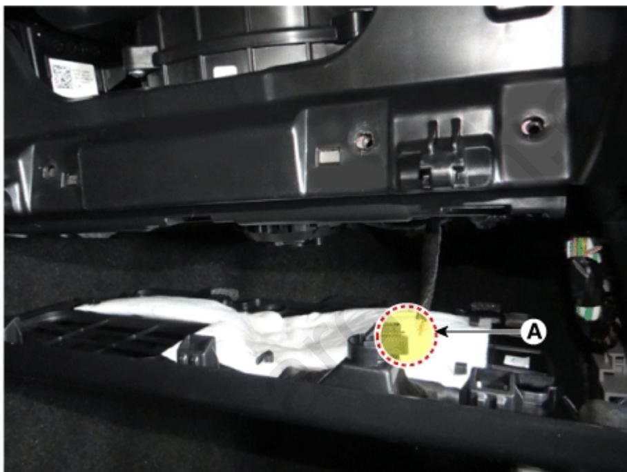
26. Separate the glove box housing (A) after loosening the mounting screws, bolts, and nuts.
