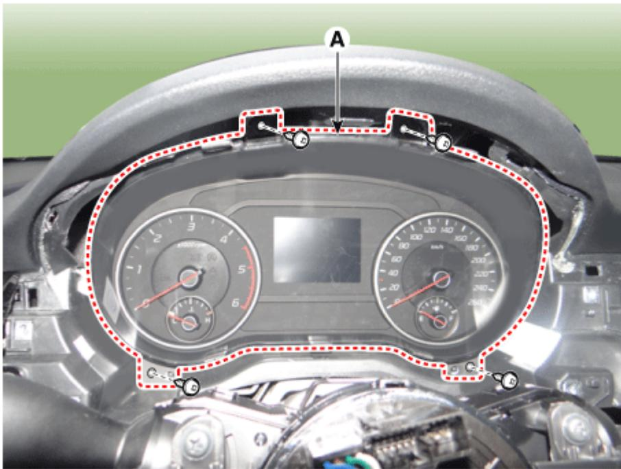
18. Remove the cluster assembly (A) after disconnecting the connector.
