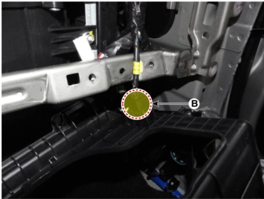
28. Remove the smart key antenna (B) after disconnecting the connector (A) and screws.
