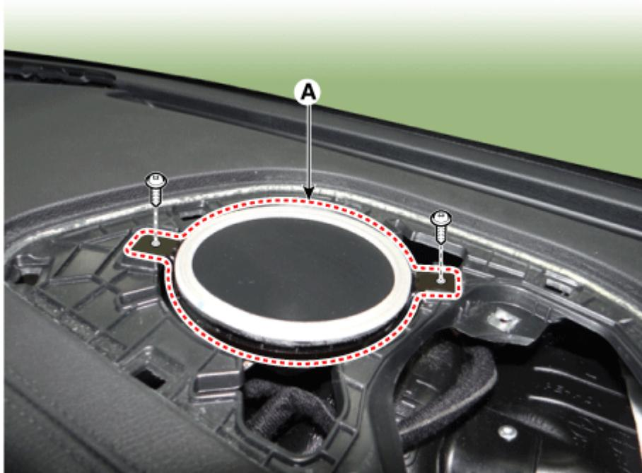
37. Remove the center speaker after disconnecting the connector (A).
