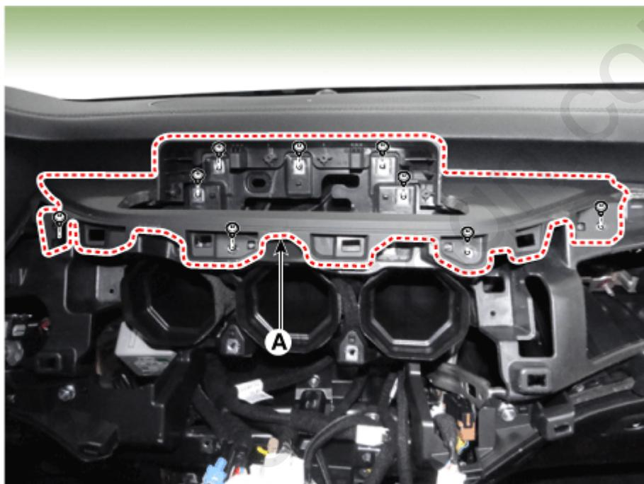
34. Separate the center speaker grill (A) by using a remover.
