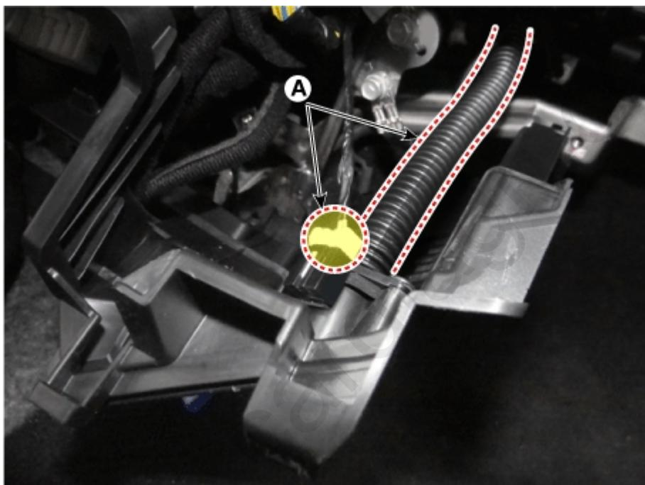
40. Loosen the passenger airbag module mounting bolts (A).
