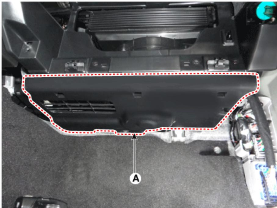
25. Disconnect the lamp connector (A) and remove crash pad under cover.
