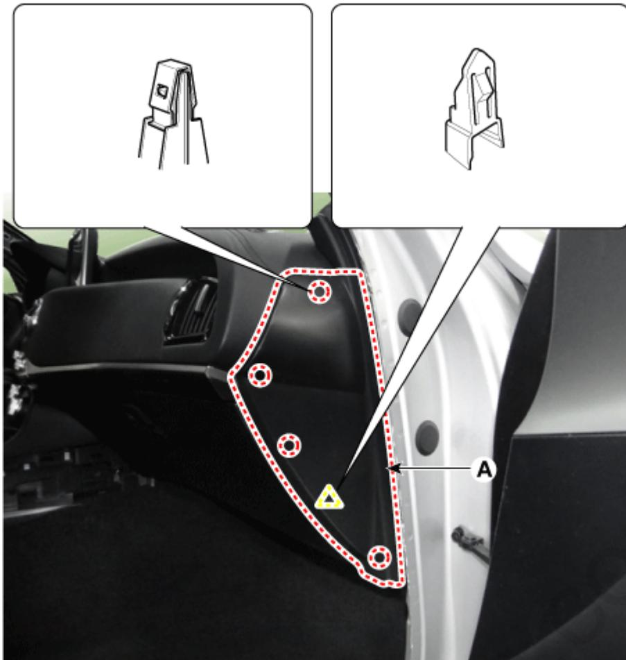
12. Remove the crash pad garnish [RH] (A) after loosening the mounting screws.
