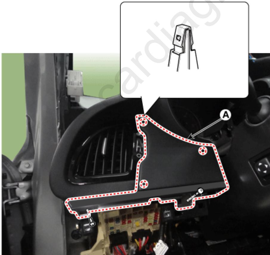
11. Remove the crash pad side cover [RH] (A) by using a remover.
