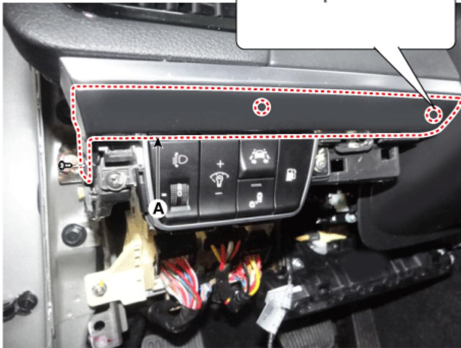
10. Remove the crash pad driver side panel (A) after loosening the mounting screws.
