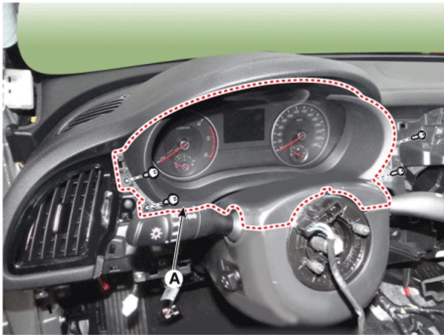
16. Remove the steering column shroud lower panel (A) after loosening the mounting screws.
