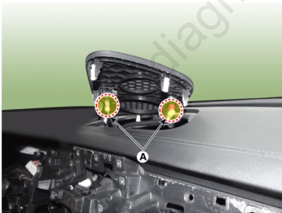
36. Separate the center speaker (A) after loosening the mounting screws.
