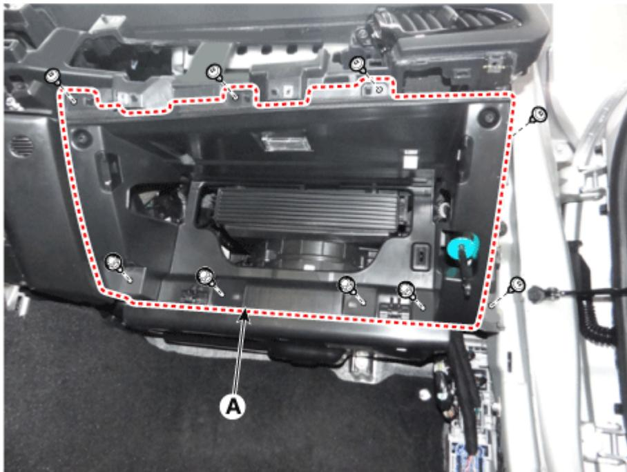
27. Remove the glove box housing after disconnecting the connector (A), (B).
