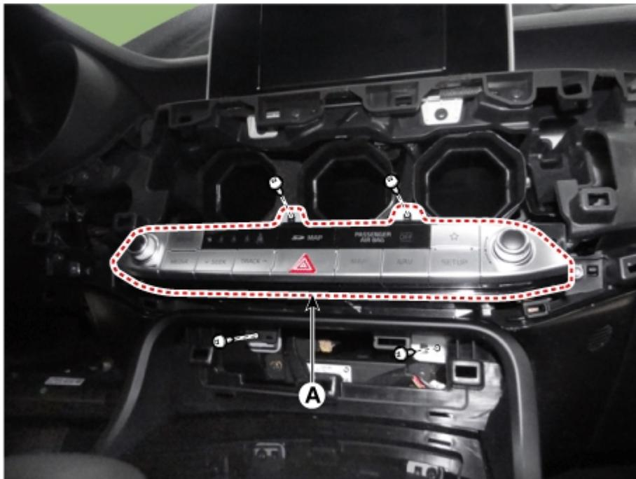
30. Remove the AVN head unit after disconnect the connectors (A).
