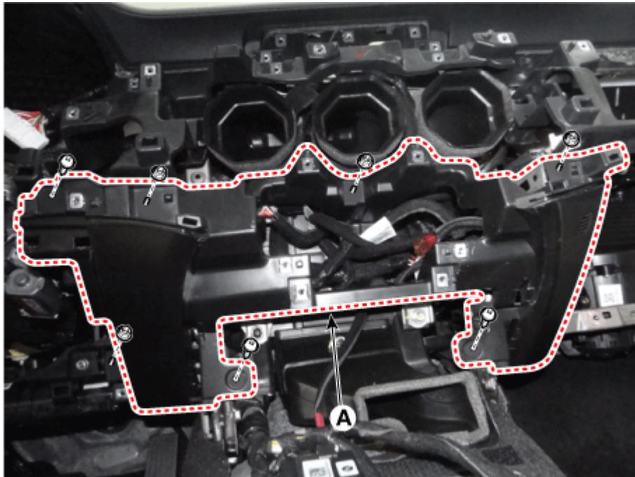
39. Remove the crash pad center lower cover after disconnecting the hose & connector (A).
