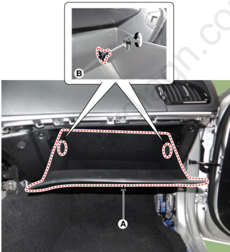
22. Remove the air damper (A) from the glove box (B).
