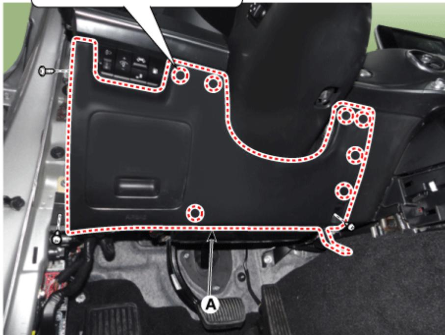
8. Disconnect the crash pad lower switch connector (A).
