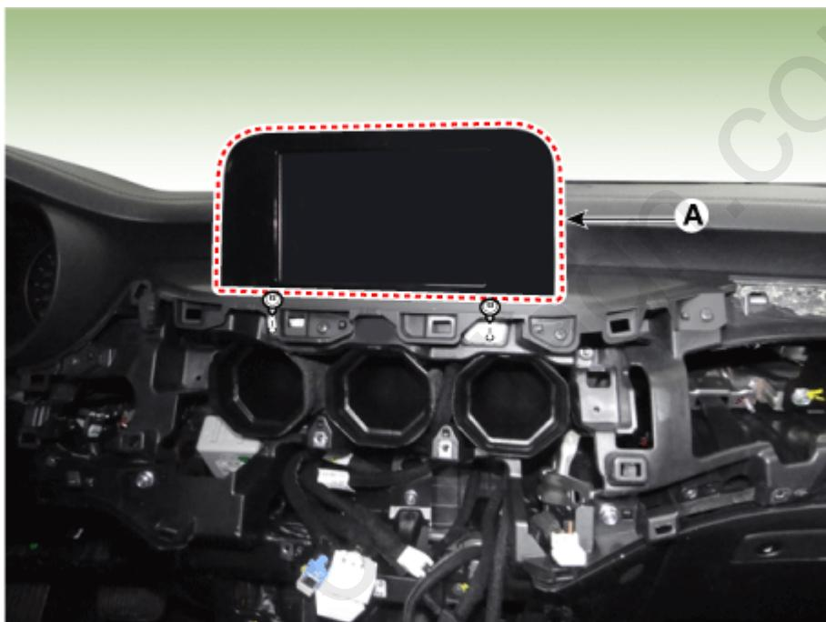
32. Remove the monitor assembly (A) after disconnecting the connectors.
