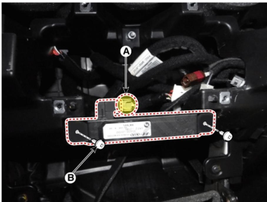
29. Separate the AVN head unit (A) after loosening the mounting screws.
