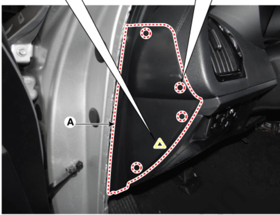
7. Separate the crash pad lower panel (A) after loosening the bolts and screws.
