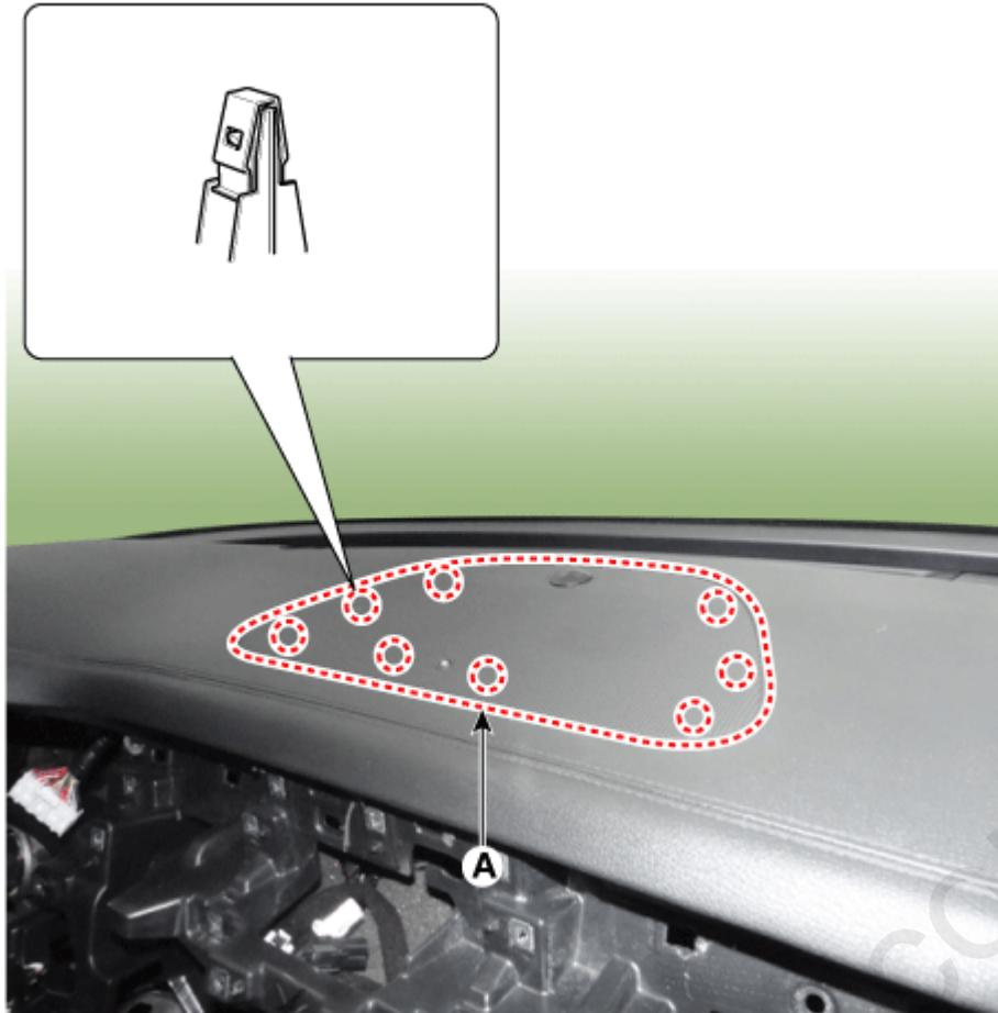
35. Remove the center speaker grill after disconnecting the auto light photo sensor & security indicator connector (A).
